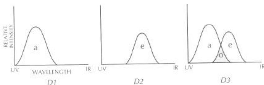
The EXCITATION spectrum of a given fluorochrome is determined in a similar manner. The emission maximum is chosen and only emission light at that emission wavelength is allowed to pass to the detector. Then excitation is induced—by means of a monochromator—at various excitation wavelengths and the intensity of the emitted fluorescence is measured. The result is a graph/curve which depicts the relative FLUORESCENCE intensity caused by excitation at the successive excitation wavelengths. (Fig. D1)
