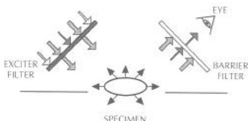
It should be noted that this is the only mode of microscopy in which the specimen, subsequent to excitation, gives off its own light. The emitted light re-radiates spherically in all directions, regardless of the direction of the exciting light.
