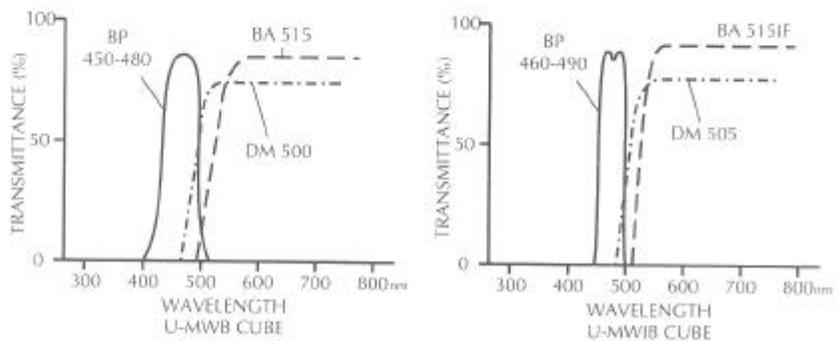
If you wish to narrow the excitation band for blue excitation, you might choose the U-MWIB cube. This cube has an interference excitation filter (very sharp slopes on either side of the excitation band) BP460-490, a dichroic mirror DM505 and a barrier long pass 515IF (interference barrier filter). The sharp slopes of the exciter and barrier filters do a better job in separation of excitation and emission wavelengths with minimum overlap.
