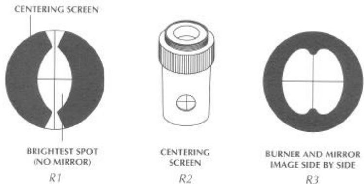
If the lamphouse contains a mirror, the mirror position should be adjusted so that the arc image in the mirror is positioned parallel and adjacent to the arc image itself (Fig. R3).
