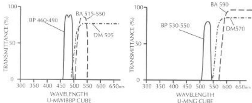
Similarly, for other combinations of multiple fluorochrome staining, the user must know the excitation-emission spectra for the fluorochromes and the transmission curves for the cubes supplied by the microscope manufacturer.
