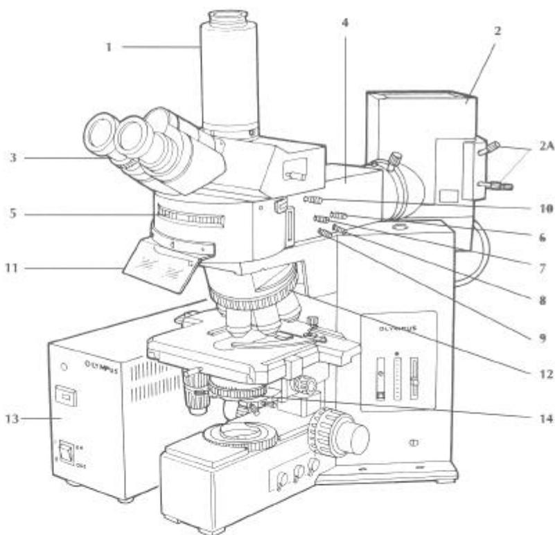
The illuminator is designed to direct light onto the specimen by first passing the light through the microscope objective on the way toward the specimen and then using that same objective to capture the light being emitted by the specimen. (Fig. J)
