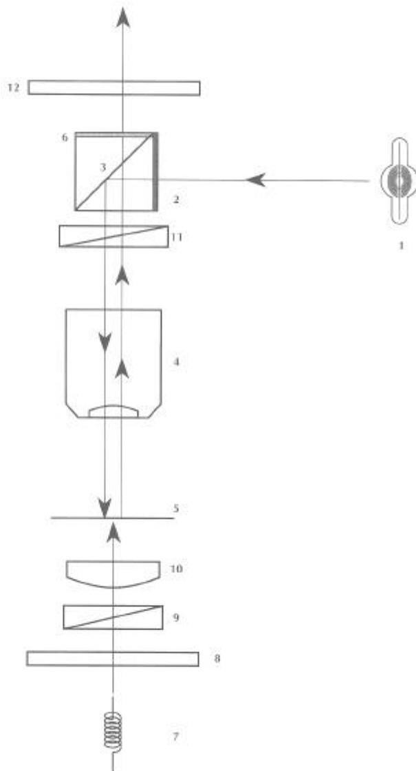
The design of the illuminator should permit the user to employ the desirable Koehler illumination, providing bright and even illumination across the field of view. The corrected condensing lenses of the system make certain that the image of the centerable aperture diaphragm is conjugate with the back aperture of the focused objective. The image of the pre-focused, centerable field diaphragm is conjugate with the focused specimen and the plane of the fixed eyepiece diaphragm.(Fig. N)
